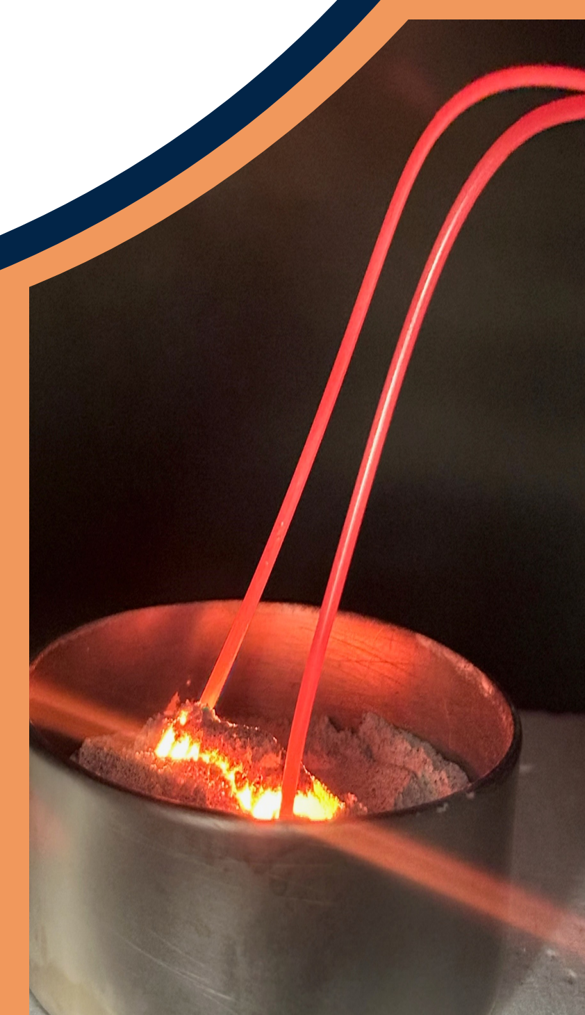
Figure 3: Lab testing of regolith melts for off-gassing characteristics under high vacuum.
